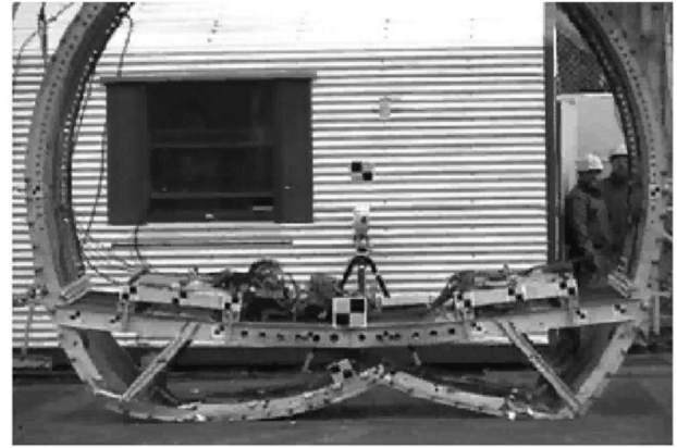
Fig. 3 Photograph of deformed Fokker F28 fuselage section.
